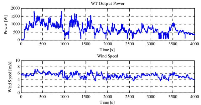
Fig. 11. Wind turbine output power and wind speed waveforms
