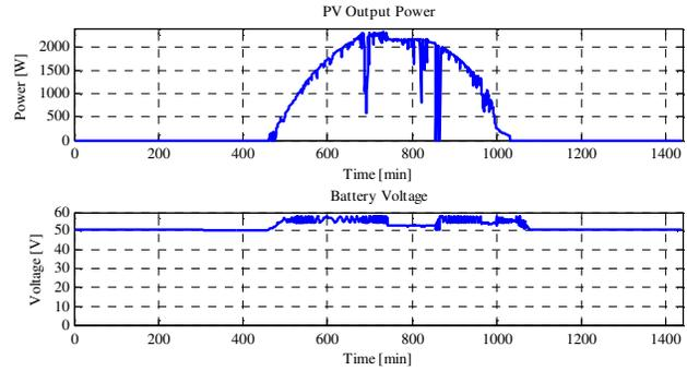
Fig. 10. PV output power and battery voltage waveforms
