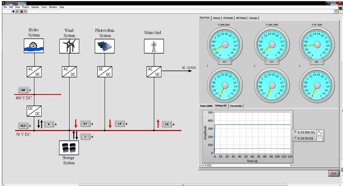
Fig. 9. SCADA User Interface
