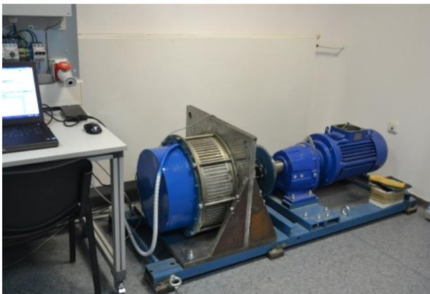
Fig. 5. The Wind Turbine Simulator
