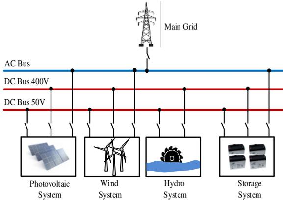
Fig. 1. Microgrid Topology
