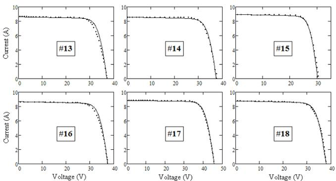
Measured and estimated I-V characteristics of six commercial PV modules [2]
