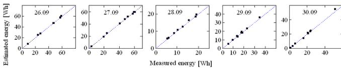
Estimated vs. measured energy delivered per hour by the PV-R system operating during September 26-30, 2012 on the Solar Platform [1].
